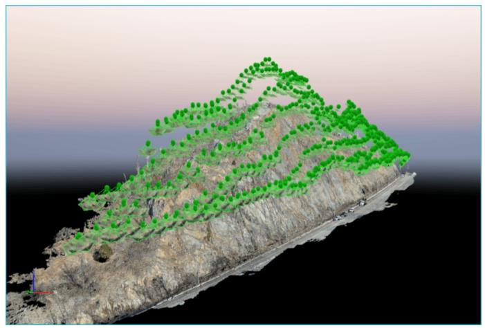
An example of a UAS terrain tracking flight model from a New Jersey project. Terrain tracking flights greatly improve model results, as can be seen in this point cloud video.-
