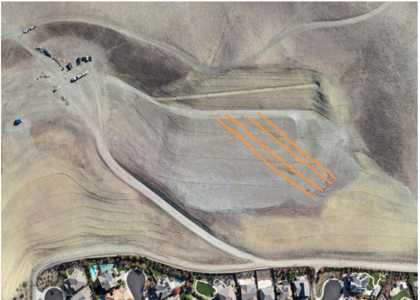
The image shows the completion of the phase 1 repair and delineates leaching sand beds (orange lines).
