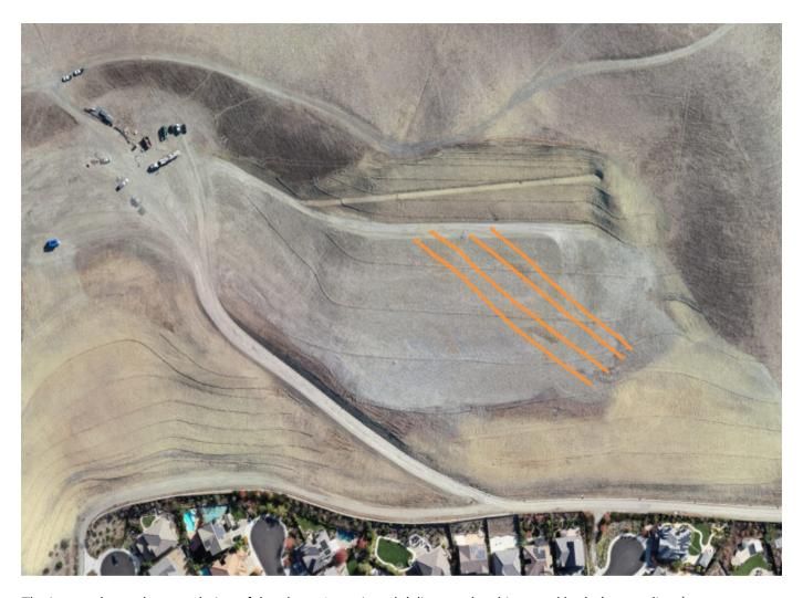
The image shows the completion of the phase 1 repair and delineates leaching sand beds (orange lines).
