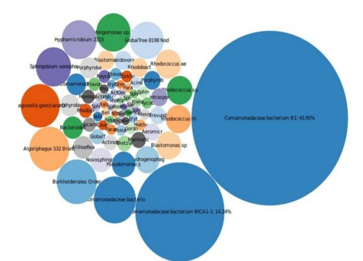
Microbial testing at this chlorinated solvent site in bedrock indicates a large variety of bacteria, some known to degrade the contaminant.
