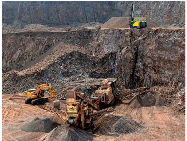
Figure 3: Aggregates can also be “manufactured” from mined bedrock deposits.
