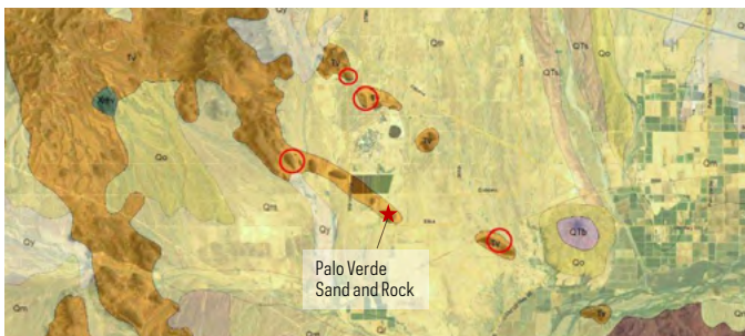
Figure 10: Active mining from a basalt unit (Tv) suggests that other basalt deposits in the area are potential aggregate sources.
