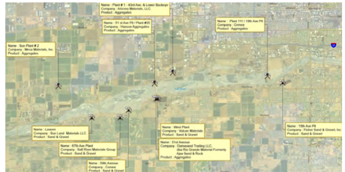
Figure 9: Overlaying mining sites on Phoenix Geologic Map shows strong correlation with recent alluvial deposits denoted as Qr (Recent Quaternary Alluvium).
