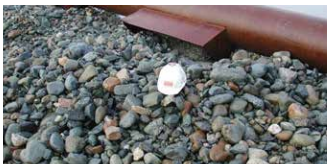
Figure 4: Gravel, cobbles and boulders from deep glacial meltwater deposits below the Taunton River. Note hard hat for scale
